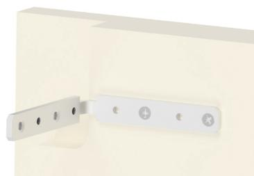
Attach bracket to carcase side using 2 x 3.5 x 13mm chipboard screws.
